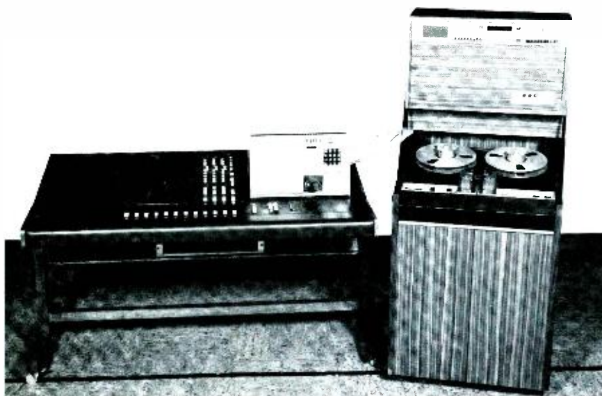
Figure 3 BBC Research Department's 10-channel digital audiotape recorder was digitally coupled to an experimental digital mixing console, based on a Plessey Miproc computer. The recorder is the forerunner of the 3M/BBC multi-channel recorder.
