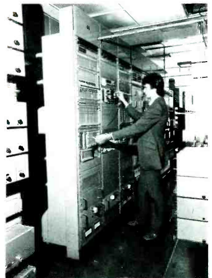
Figure 2 This BBC designed and manufactured 13-channel digital audio multiplex encoding equipment, including a complete reserve set and monitoring facilities, forms part of BBC Radio's distribution network throughout the UK.
